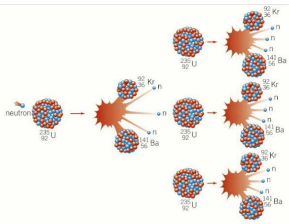
▲ **Figure 3** An uncontrolled chain fission reaction
