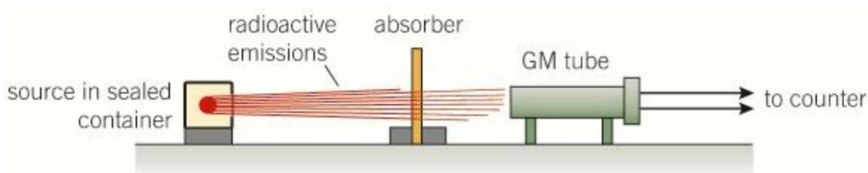
▲ **Figure 3** Experimenting with radiation and different absorbers
